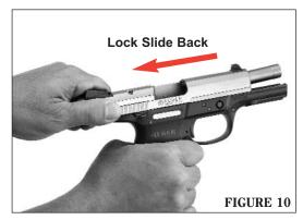
3. Keep upward pressure on the slide stop to prevent forward movement of slide. The open slide is under strong spring tension and could injure fingers if allowed to slam shut. Insert finger (or another non-metallic object such as the eraser end of a pencil) through the top of the slide and push the ejector downward and forward until it locks in its forward position. (See Figure 11.) This will permit forward movement of the slide off the front of the frame.
